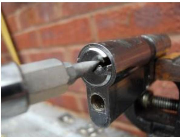
5 chambers successfully drilled you can now rotate the plug in the direction needed to open the door. It's of paramount importance you drill NO FURTHER than the last pin chamber otherwise you risk damaging the cam assembly that has the notch attached to operate the Multi Point Locking Gearbox.
