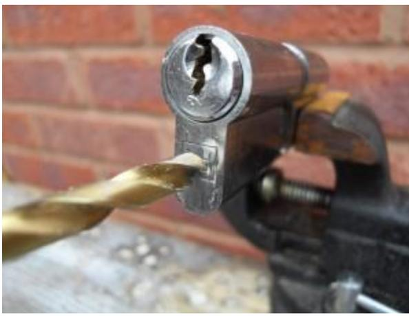
With the dimple in place I'm going to start drilling confident that the drill's going to stay firmly centred on my dimple mark and not wander or skid off.
