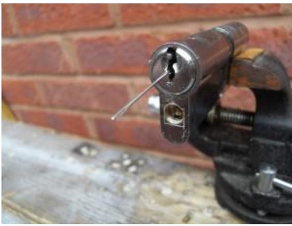
I'm using a sewing needle to push the pins down into the drilled hole. It's an everyday item that most people have lying about.
