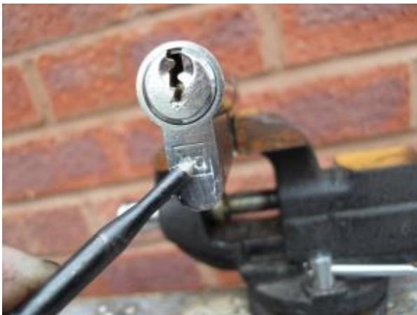
I'm going to make a dimple with a centre punch in the area indicated. A few light taps with a punch and hammer should do it. If you don't have a punch a steel nail makes a good substitute.
