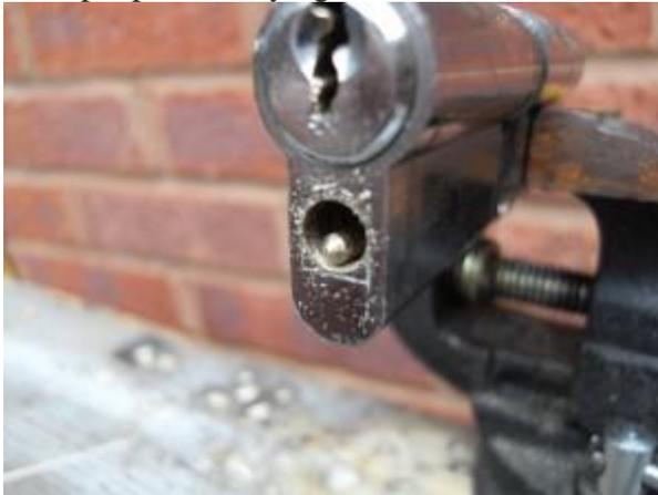
Here's a key pin that's been pushed down into the drill hole with the needle, you should get a feel for how far you have to drill in to reach each chamber. You need to stop drilling at chamber 5 make 100% sure all the pins and debris are removed then check the lock to see if it'll open most times it will, if it won't drill very carefully to see if there's a 6th chamber if there isn't you haven't fully removed all the debris from the first 5 chambers.
