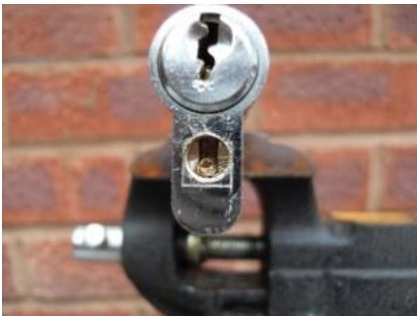
The drill bit has now encountered the first pin chamber, when this happens you'll hear the drilling noise change more to a screeching type of noise and you'll feel a jolt down the drill. It's important now that you count the pin chambers as you're drilling through them. Also I recommend you clean out each pin chamber as you come to them.
