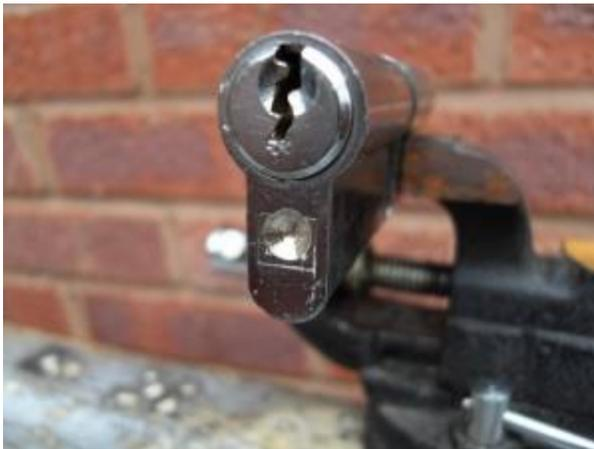
The drill hole is nicely centred in the section that houses the pins. Make sure your drill bit is nice and sharp so that the drilling edge is easily removing the brass without pushing too heavily on the drill bit.
